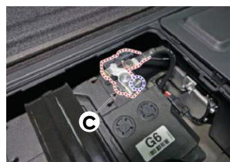
4-3. Turn the ignition switch OFF and disconnect the auxiliary 12V auxiliary battery negative (-) terminal (C).
